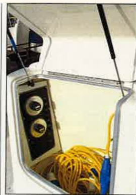
Above: one of the lockers set in the transom coaming houses battery switches and a shorepower cable.
