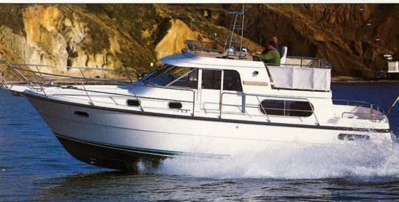
Left: the 37 provides ample space for enjoying the open air, with an aft cockpit augmenting the flybridge. Above right: design features include the mounting of guardrail stanchions on the outside of the gunwale, rubber D-fendering all around and a break in the pulpit, with handrails, enabling you to step ashore from the bow.
