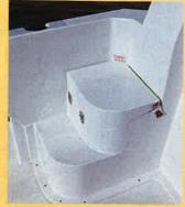
walk-through gate or integral bathing platform. A stainless steel and teak arrangement is available as a bolt-on extra, accessible via a set of steps over the coaming.
