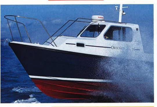
raded with a full cruising eventory, and our test figures edicate that a fast cruise setting of 500rpm should give 24-25 knots.
