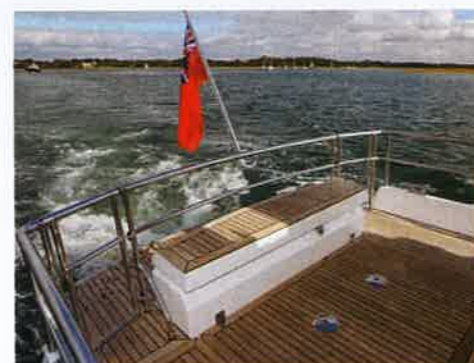
Solid guardrails rather than coamings work well
