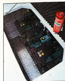
Above: located under a hinged hatch below the aft cockpit, the engineroom has an aluminium treadplate and eggbox soundproofing. Bottom: all instruments are within easy reach at the helm, although the power-trim switches are awkwardly placed behind the wheel.
