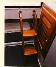
above The cuddy cabin has stowage behind the steps, a separate WC and a fixed double berth.
