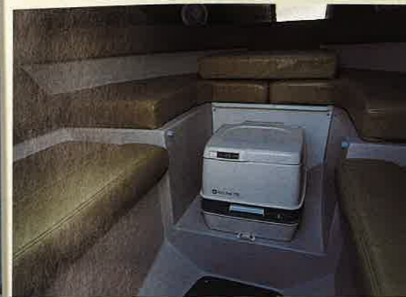
toilet A portable loo is housed under the forward berths.
