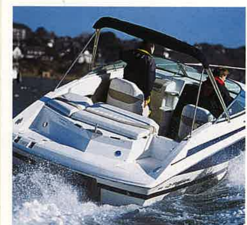
bathing platform Of a decent size, the platform has an L-shape which naturally leads you through to the cockpit via a transom gate.
