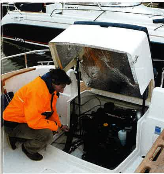
above The enginebox lid lifts on gas struts.
