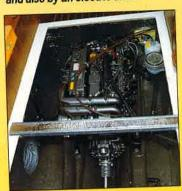
and the builders are right not to be tempted to overpower it. The 85hp Yanmar installed in our test boat fits the bill perfectly, giving a top speed of nearly 16 knots and a cruising speed (300rpm down on its rated 3800rpm) of just under 14 knots.
