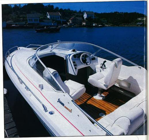
for various odds and ends, with storage for fenders and other bulky items under the bench settee and beneath the wood veneered sole. The battery box and main 12V isolator together with a manual bilge pump and fuel cut-off lie under the former.
