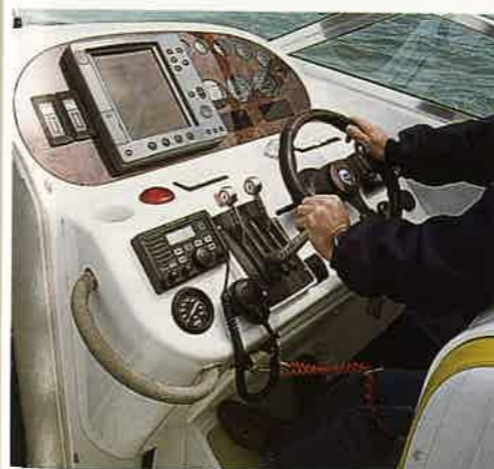
console Trim tab controls and the rocker switches are above the wheel and throttles, whilst engine gauges are set in an upper level against a burr wood backing, with the Raymarine navigational package.
