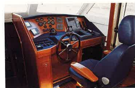
inside helm Owner Len Wilcox did not want a fixed helm seat, so a movable arrangement on a sliding carriage was devised. One by-product is clearer access through the door to the starboard side deck.
