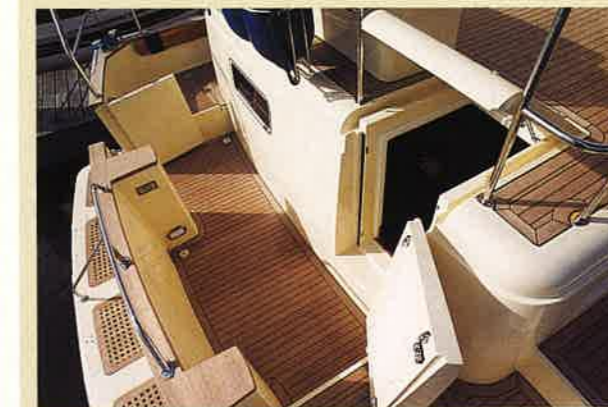
stern A transom gate gives access from the bathing platform to the decks, and to the aft cabin, via a hatch in the quarterdeck.
