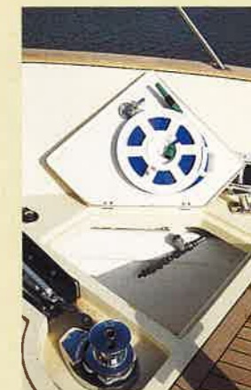
foredeck This is mini-ship style, with large bitts and enclosed fairleads. A freshwater wash-down hose is incorporated in the locker.
