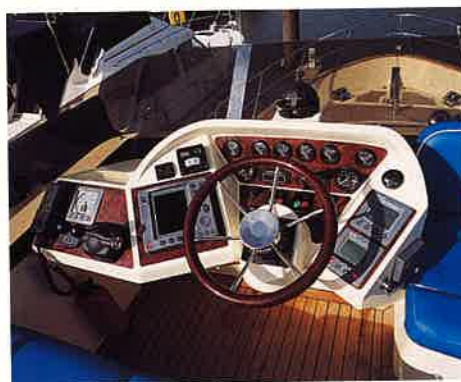
outside helm The two-person seat has lifting squabs, and the console is ranged around the skipper to good effect. There is plenty of room for fitting additional electronics beyond the standard package, which includes an autopilot and VHF.
