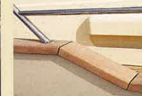
side decks The raised gunwales are topped with teak, and 12in (30cm) midships bitts.
