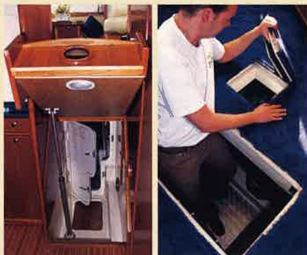
above Access is by hydraulically raising the galley stairs or removing hatches in the sole.
