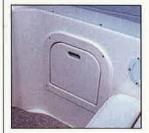
Above: a neat step which folds down from the starboard coaming offers a handy leg-up to the side deck. Below: to port, the function is performed by a fixed part of the moulding beside the wet-bar.
