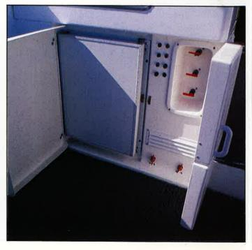
A door to the back of the port settee gives easy access to the fuel cut-offs, master circuit breakers and battery switches — a neat idea. The optional second fridge also finds a home behind a second door here. Far left: starboard side of the sociable lower cockpit area. Above left: the comprehensively equipped galley to port. Above: the saloon looking towards the master cabin forward and right: a closer view of the same cabin.
