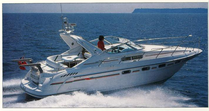
tunnels for the Statesman's shafts, the shape of the rest of the hull, including the integral bathing platform and the incorporation of the anchor stowage in the forebody, appears identical.
