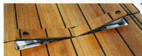
Hidden chocks spring up from the bathing platform
