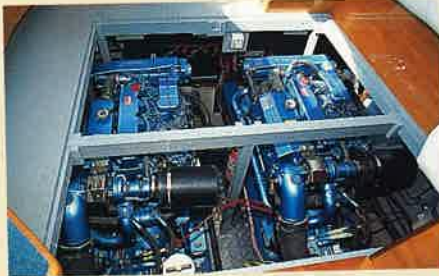
above A single engine installation has space around it; twin Nannis have a treadplate in between.
