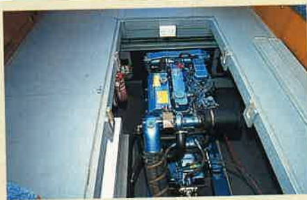
above A single engine installation has space around it; twin Nannis have a treadplate in between.
