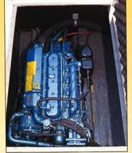
separator located on the forward bulkhead. With everything well clipped and secured, and the whole enginespace gel-flowed for ease of cleaning, it is a tidy installation.
