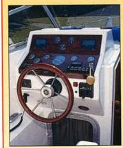
engine gauges, there is a helm indicator, depth-sounder and log, so all the basic requirements for river and estuary cruising are catered for. The throttle is located on the outboard coaming, to the skipper's left hand, while the wooden wheel is vertical.
