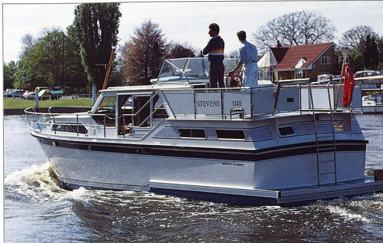
shotblasting to clean weld areas after construction. The finish is a Sikkens single-pot epoxy paint system, with International Interguard employed below the waterline.
