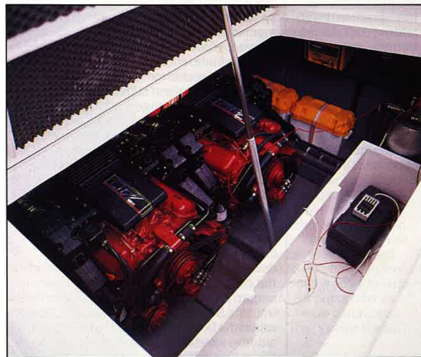
Top: handling and ride were superb. Above: 660hp fits snugly under the sun-lounger, with access still good.
