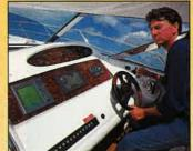
includes radar, autopilot, GPS and VHF, while the engine gauges are set in a veneered panel topped off by a wet-card compass. A console return to the skipper's right provides a landing for the throttles, and the ready-use switches are rafted to the left of the angled leather-trimmed
