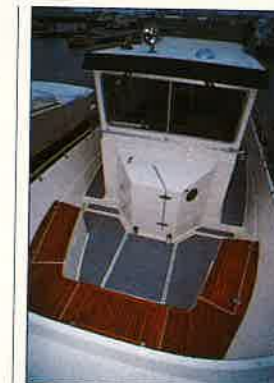
Above: the forward cockpit offers moulded U-seating and a large lazaret under the sole. Below left: access to the sleeping cabin is via a door which also acts as part of the saloon seating.
