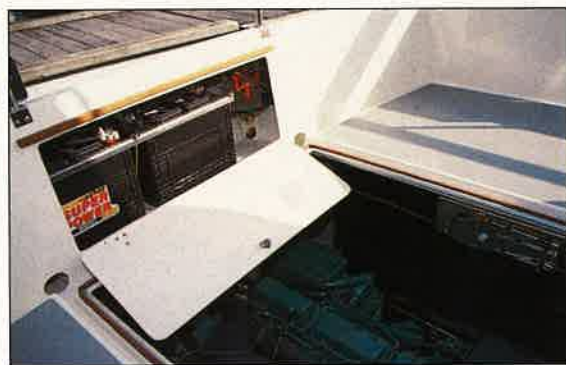
Above: plenty of handholds help out at the exterior helm, not such an insecure perch as it might seem. Left: the engine, a single 230hp Volvo diesel on our test boat, is found under a full-size hatch in the aft cockpit, with the batteries housed in the transom coaming.
