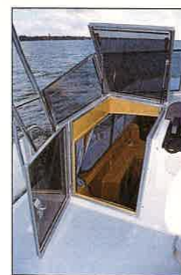
Above: you enter the Veba's accommodation via a hatch which looks ungainly when raised. Top left: the open-plan layout features no interior helm or separate forward sleeping area. Below left: the aft cabin has a good array of cupboards and drawers. Top right: the galley straddles the full beam of the boat, with the cooker and sink to port. Right: a single pedestal seat faces a neat but unprotected console.
