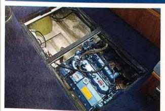
A double hatch in the saloon sole opens up a roomy enginebay. All sides of the single diesel can be got at, and access to the service points could not be better, with filters, seacocks and batteries all easily to hand.
