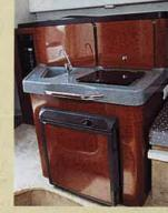
galley A sink and a single-burner stove with a hinged top are set into the moulded worktop, with a fridge and a locker underneath.
