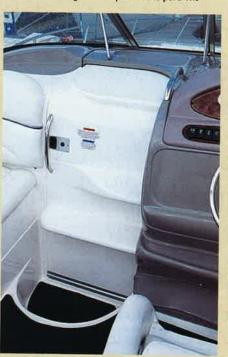
access Steps set into the sliding cabin door moulding facilitate access forward through the opening windscreen.
