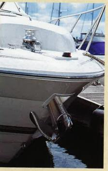
foredeck Our test boat had a tidy through-deck fitting for the anchor and windlass, with remote operation, but this is an optional extra.
