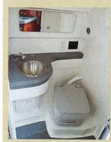
toilet The moulded compartment has an inset stainless steel sink, and the tap has a wanderlead to double as a shower.
