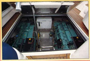
plenty of space to get right around both engines. This makes it easy to carry out day-to-day checks, service the water filters and fuel/water separators located on the forward bulkhead, and even get at the shaft logs which, due to the V-drive arrangement, are beneath the
