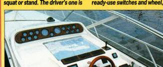
also adjustable fore and aft. A simply but effectively laid-out console has engine instrumentation set furthest away, a perspex chart area immediately in front of the
