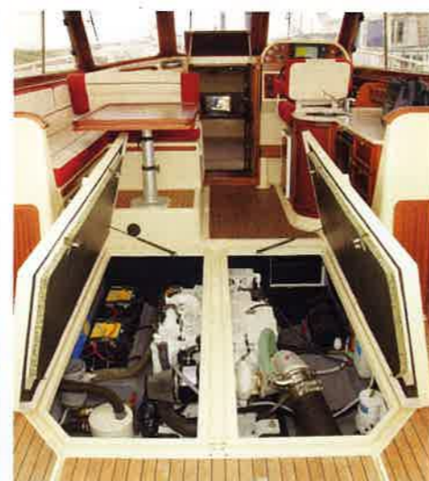
Single engine makes access straight-forward
