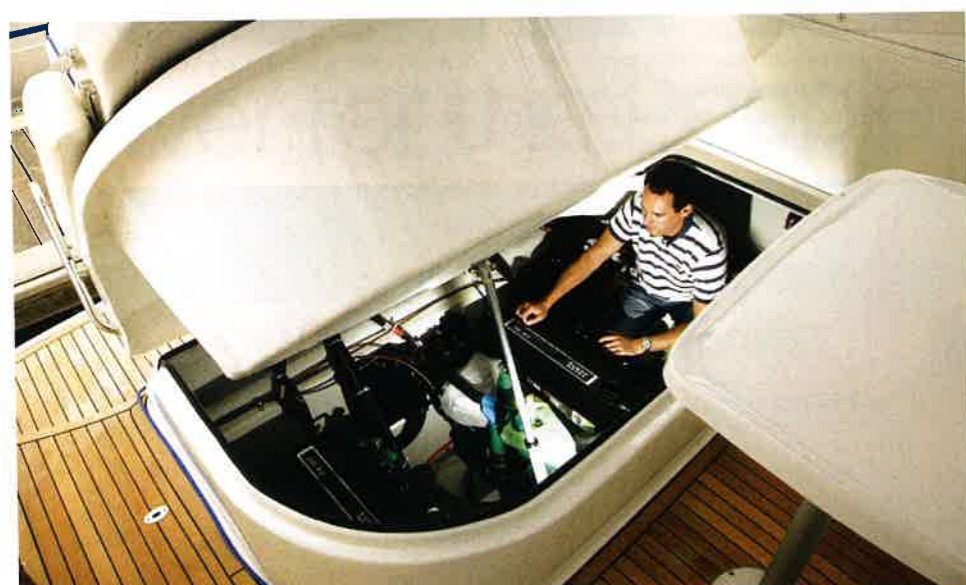
With no ladder fitted, getting into the deep engine bay could be easier. Once inside there is decent space
