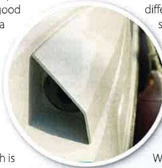
Top side air scoops feed the step hull
