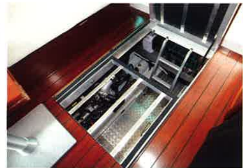
above You can crawl on a treadplate between the engines. A ladder and automatic light help you down.
