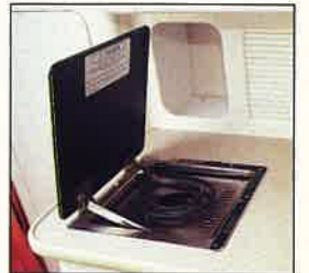
Below: the neatly covered electric/alcohol hob in the galley has a single burner. Bottom: the toilet/shower compartment opposite is both roomy and practical, with moulded lips on the countertop and plenty of stowage.
