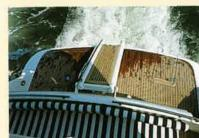
The platform's depth, following the current trend, is generous enough that it can be used to land a tender. Two inset hatches give onto a wet locker and boarding ladder with teak treads.
