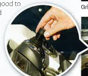
Volvo's IPS joystick controls come as standard on the Targa 44
