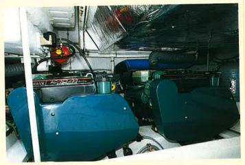
In this way, access to and around the engines is wholly adequate for most maintenance jobs, such as day-to-day checks and filter changes. There is sufficient room between and down the sides of the engines to get at everything, the only exception being the port engine's dipstick, but this has a separate hatch over it so that it can be more easily inspected.
