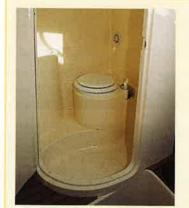
The WC is constructed of moulded units which incorporate the sea toilet and wash basin, but offer little stowage. A shower, which would be a standard fitment for most builders, is missing here.
