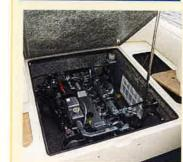
The centre section of the cockpit's aft sunbed/settee hinges up to give very good engine access. There is no power lift or gas strut, but a simple pole to support the engine cover in the raised position.
