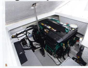
Clean, tidy and accessible sums up the smoothly gel-coated engine bay. Access is via a large hudraulicallu powered engine hatch that takes the dinette table with it. There is no secondaru inspection hatch but the main one can be opened manually. The centrally mounted single Volvo D4 engine, batteries, wiring and ancillaries are all tidily installed and veru easu to get at for service checks.
