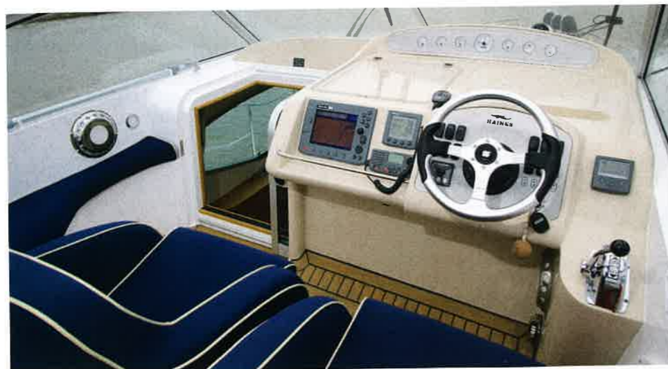
Two bucket seats at the smart helm slide back and forth, and swivel round to face the settee aft
