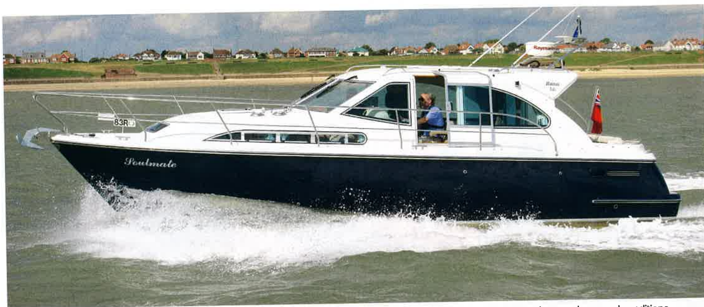
At 13 knots the Haines runs at a low angle of trim, giving good forward visibility, while the topsides knuckle keeps the spray down under normal conditions
