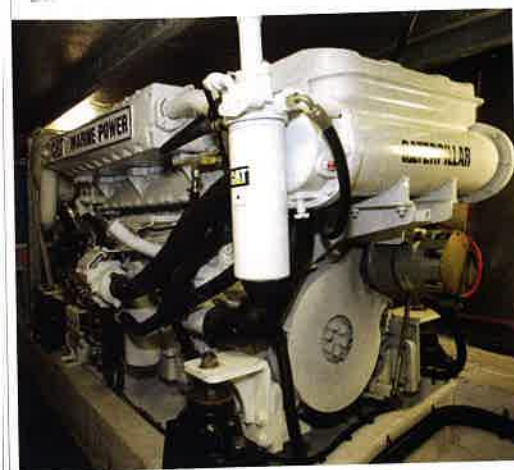
above The twin 700hp Caterpillar diesels are accessible via a walk-through door. above Practical features include a utility room and safe, wide side decks.
