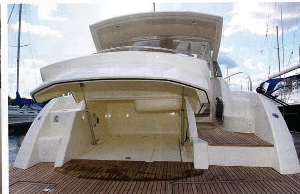
The teak deck runs into the tender garage, which makes the removal of a dinghy that much easier
