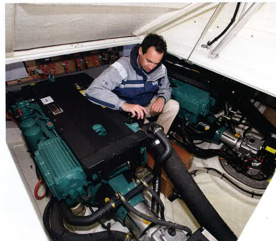
There's plenty of space above and to the sides of the twin IPS drives in this well-protected engineroom
