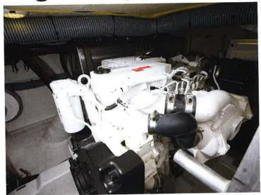
A hatch in the cockpit floor directly above the engines makes initial access easy, but the off-set tread ladder and narrow gap between the motors restricts operating space once inside, the ladder itself blocking access aft. You wouldn't want to spend much time down here when the engines
