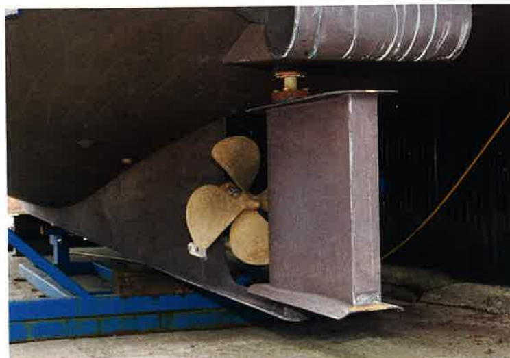
The keel helps protect the prop and the unusual, but highly effective, rudder
