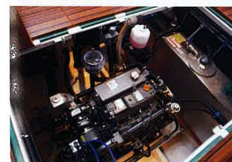
The 75hp Yanmar is tucked beneath the saloon sole
