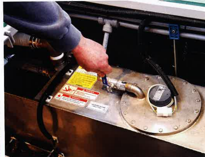
There is a freshwater flush built into the standard holding tank
