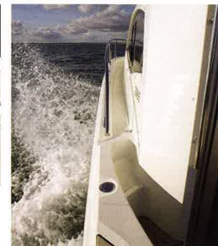
Raised gunwales improve safety on side decks
