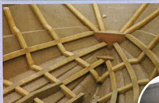
Foam stringer system before being glassed
