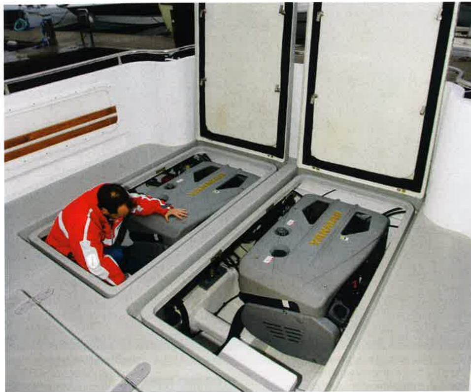
New Yanmar diesels look suitably clinical in the immaculate bay. Tall hatches need some gas struts
