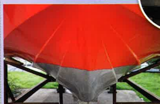
Unique spray rails create lift and cushion the ride
