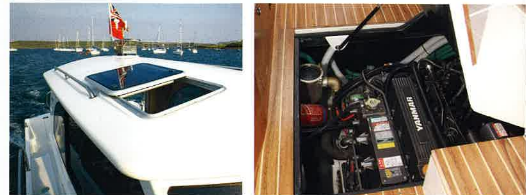
above Both side decks are wide and safe, and the engineroom hatch is supported by a gas strut.
