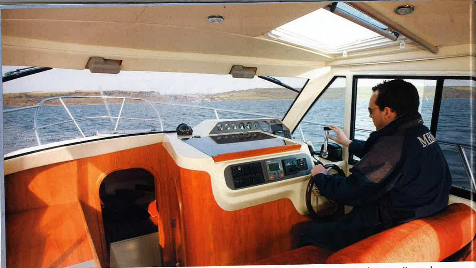
above The helm station is one of the areas that have benefits from design tweaks. There is space for two people, and a chart area on the console.
