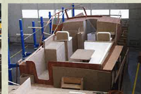
The original concept layout for the 25.9 was done using cardboard and plywood
