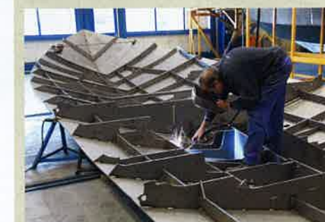
A Linssen employee gets to work on the steel hull of a future 29.9
