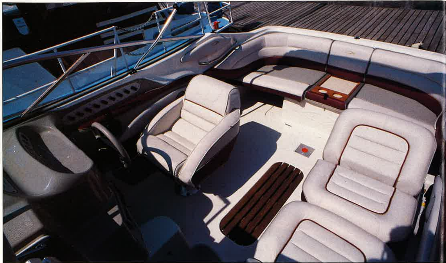
Above: the well bolstered bucket seat at the helm is almost an armchair. The back-to-back seats opposite can be folded down into a sunlounger. Below: the console is in grey rather than white, to cut down on glare.
