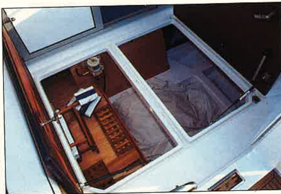
Left: hatches on gas struts open from the cockpit to the lazaret, which has wooden tops covering the steering gear and fuel tank, offers lots of space for stowage, and allows access to the fuel separator, inlet strainer, calorifier, stern gland, seacock and gearbox.
