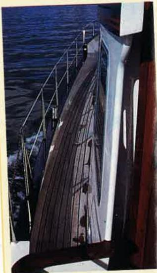
gunwale to step over. Handrails along the coachroof also help to make the 18in (46cm) wide side decks safe for crewing duties, and you are really enticed to use the whole deck area even while underway.
