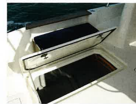
Two hatches give access to the bilge lazarette
